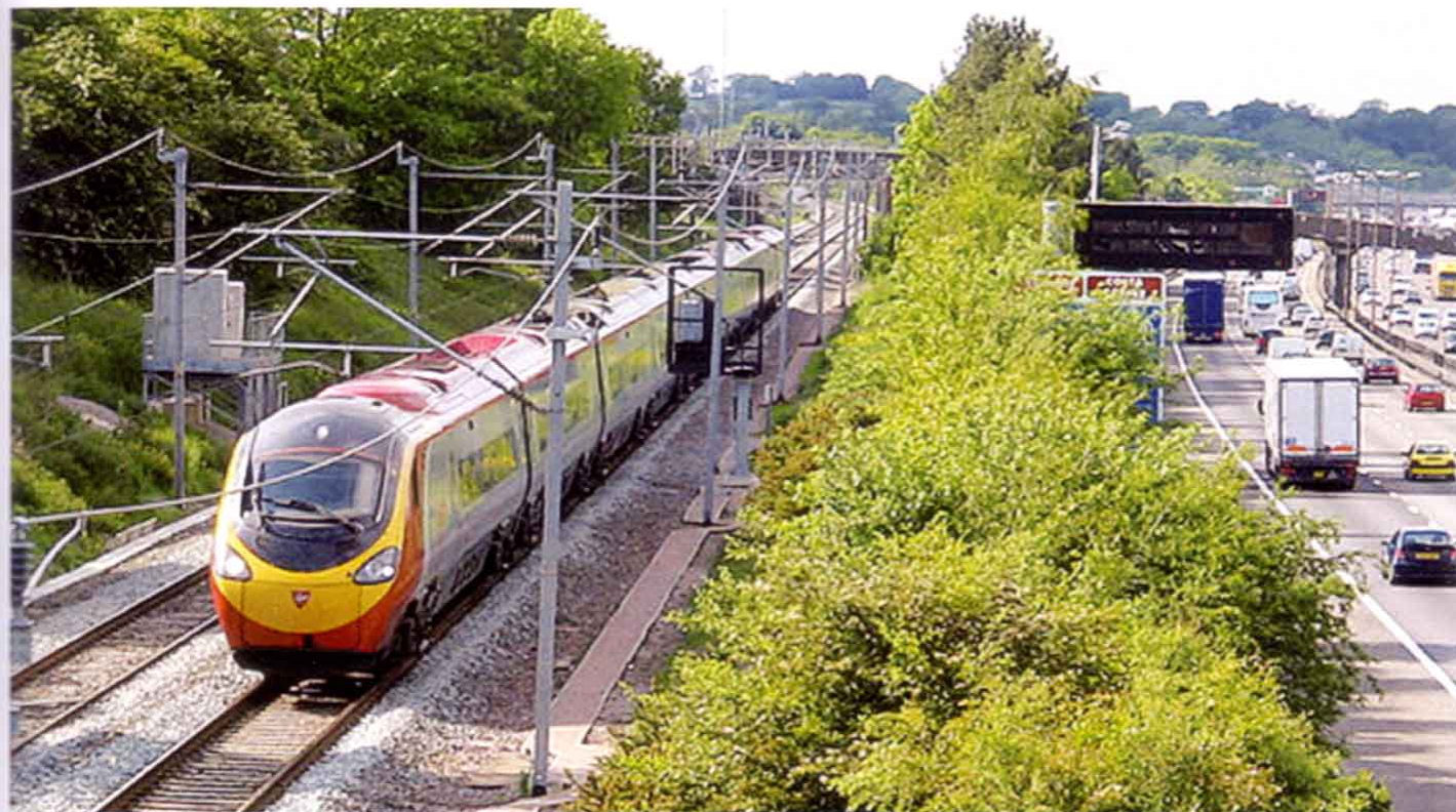
Tilting train technology developed by Fiat Ferroviaria (Pendolino) was successfully adopted by Virgin for the UK West Coast main line
