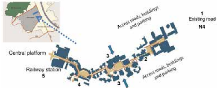
FIGURE 4 The first phase pedestrian spine. The eastern starting point is the existing N4 road (1), followed by a string of public spaces and passages through buildings, indicated by dashes (2). The diagram shows the location of access roads and car parks. The arrows indicate the vehicle underpass and parking below the “Place des Sciences” (3). The public spaces have various shapes and the alignment of their street access is either perpendicular or tangential to that of the spine (4). The sub-surface railway station (5) marks the beginning of the underground platform (see figure 6).
