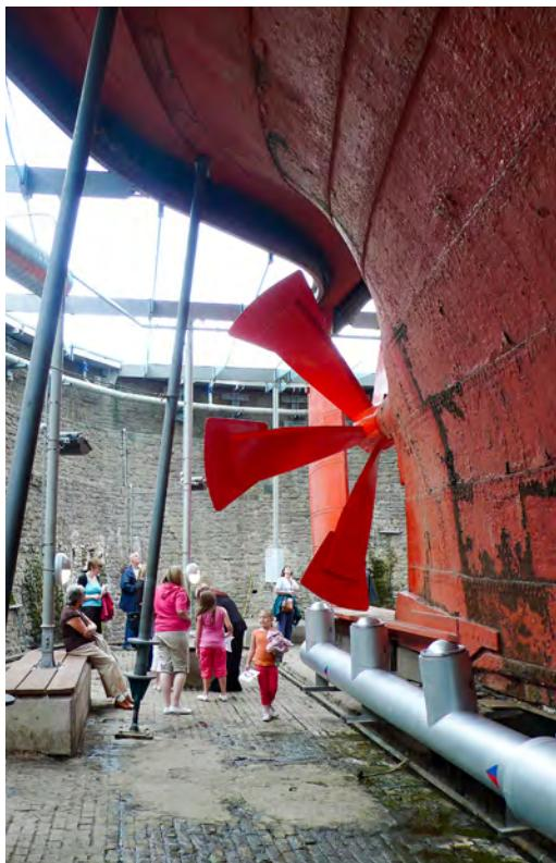
*Above: Below the waterline, replica of the vessel's original six-bladed propeller*
