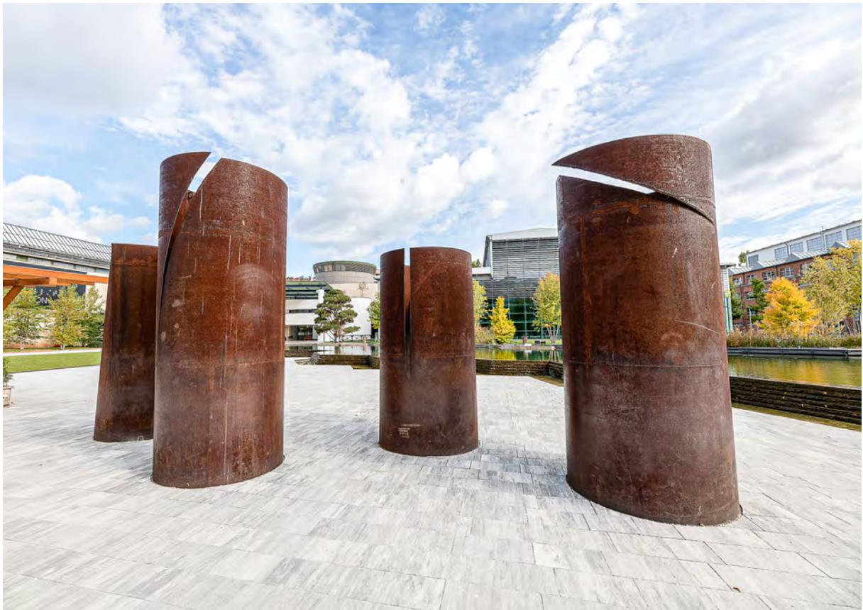
*Contemporary sculptures near the water feature; the pipes in Corten steel provide ventilation for the underground car park*
